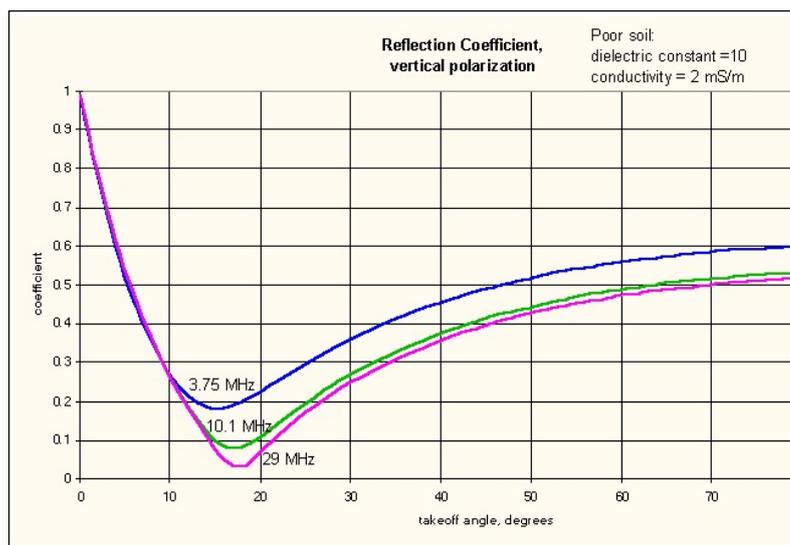
Notice that, at 10 to 25 degrees, the ground reflection is very weak. It also is shifted 90 degrees in phase from the incident ray. Therefore, radiation from the grasswire, off the ends will be about the same as if the ground were not present.
