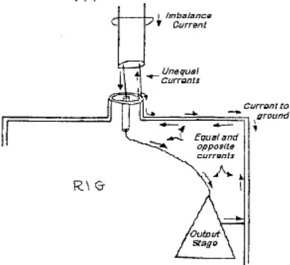
**Fig. 4 – When the rig is connected to ground, a third conductor in parallel with the right side of the feed line is introduced. This causes an imbalance in both coaxial cable and twin lead feed lines**
