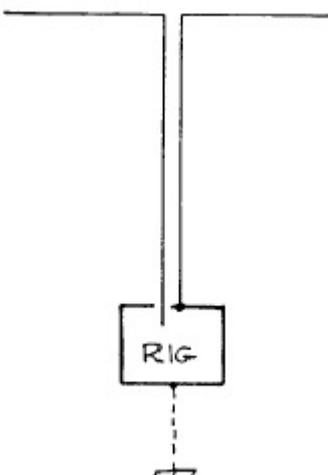
by the broken line, we've again provided a third conductor in parallel with the right side of the feed line, and the same problem occurs as with the coaxial cable (see Fig. 4). So either type of line is unbalanced if a direct path to ground is provided from one side, and both can be a balanced, non-radiating line if the imbalance current is eliminated.
