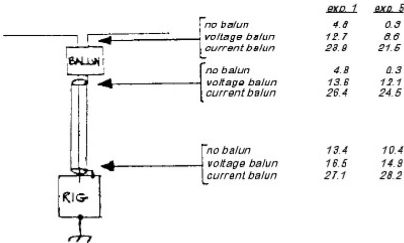
Fig. 8 — Setup and results of experiments 1 and 5. Numbers are measured
