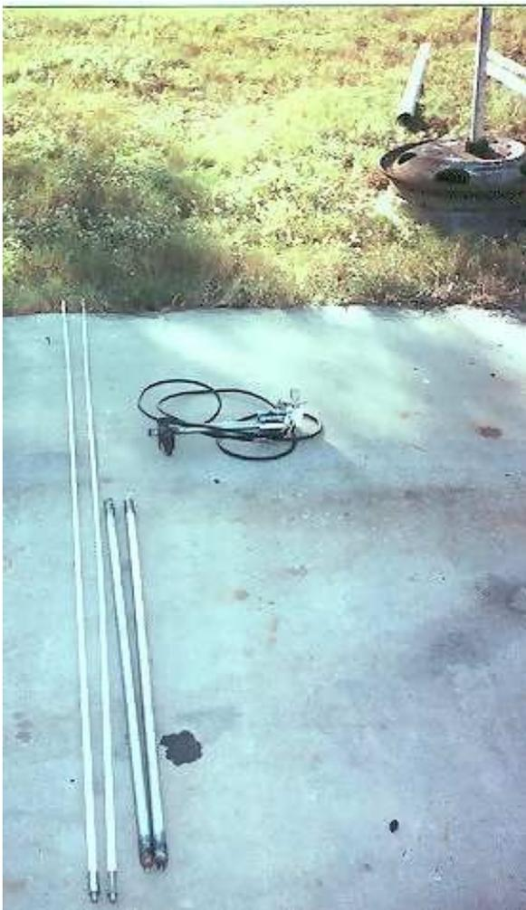
*Antenna shown broken down for field day.
