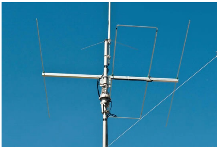
The 3el 6M LFA built by Chris, M5LRO - Pawsey stub and thru-boom mounting also, well done Chris!
