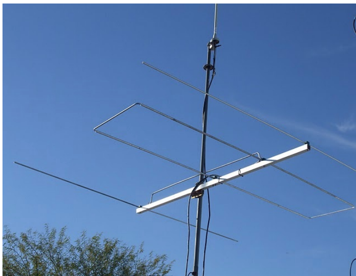
The 3el LFA for 50MHz at AD6D
